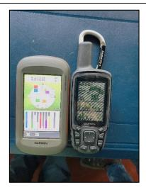
**Image 6.** Verification in the measurement of geographic coordinates from the two equipment to be used in the field. A new GPS is used as a reference.
