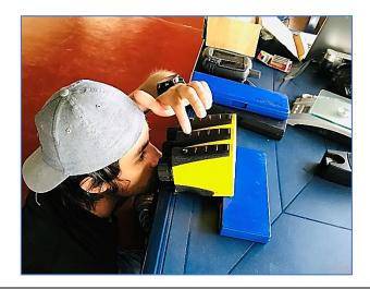
**Image 5.** Identification of errors in the calibration of digital hypsometers. The process is carried out by placing the instruments at different angles and in a flat area, checking each time the equipment to be used marks the same measurements with respect to the reference instrument or base equipment.
